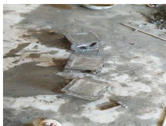
(fig 2. Casting of cube)
